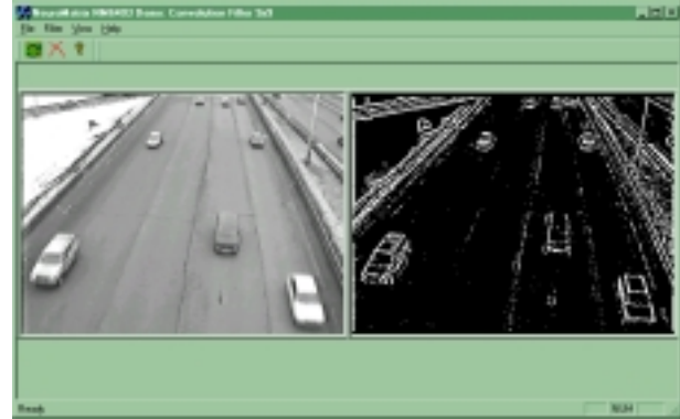
Fig. 2 Edge Enhancement with Convolution
